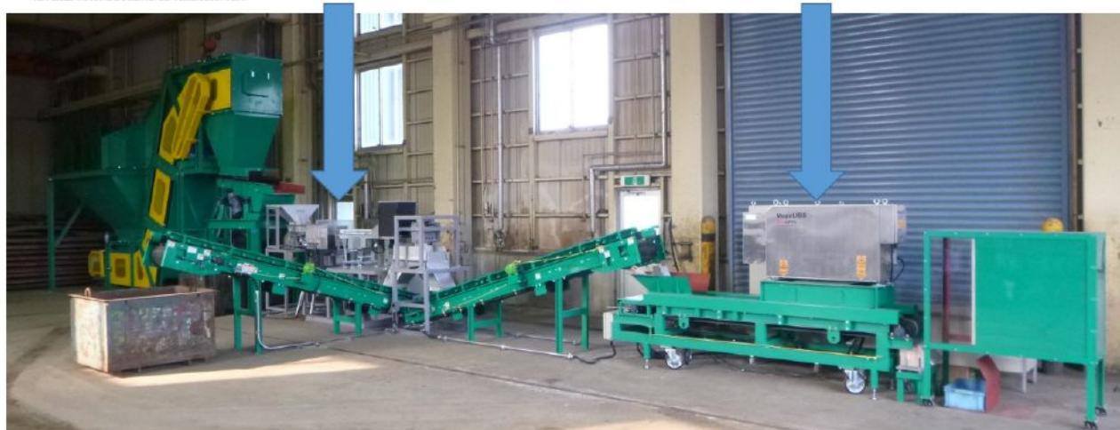
LIBS prototype sorter is made by Pellenc ST Japan
